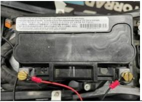
Connect your accessories to the LB-2Wire output using the 'Lever Lock' terminal output. \***Note** the **Orange** Lever Terminal is positive (+12V) and the negative (-) Lever Terminal is **Blue**.
