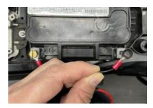
Find a suitable mounting location for the LB-2Wire. This is often under the seat. Once a location is found, secure with supplied cable ties using the holes in the 'ears' of the box and route the LB-2Wire loom to the battery area of the motorcycle.
