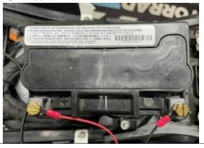
Connect your accessories to the LB-2Wire output using the 'Lever Lock' terminal output. \***Note** the **Orange** Lever Terminal is positive (+12V) and the negative (-) Lever Terminal is **Blue**.
